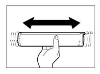
**5** Holding the toner cartridge lever, insert the toner cartridge slowly into the machine as far as it will go.
